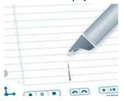
Scrubbing refers to dragging your smartpen across the paper. The contents on the display moves and scrolls in the same direction and at the same relative speed as the movement of your smartpen.
