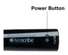
As the smartpen starts up, the display shows the words **Livescribe** and then **Starting...** After startup completes, the display shows the time.
